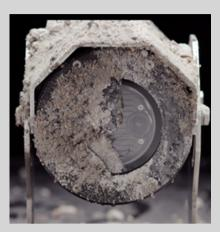
The ToughEye is a low cost & simple blast hole drilling safety and awareness system. For placement in dirty, dusty and greasy locations to get clear vision.
