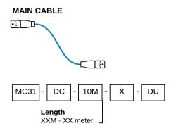
Main cable used in all ToughEye installations. Available in: **3m, 5m, 10m, 15m, 20m, 22m, 25m, 30m** lengths
