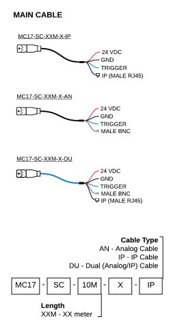
Main cable can be used in all ToughEye-1700 installations. The analog cable includes a 75-ohm coaxial cable for CVBS transmission. The IP cable includes a shielded Cat-5e cable for 10/100 Base-T signal transmission.
