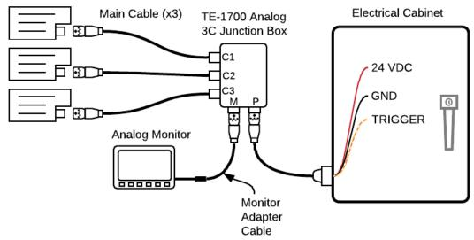
**Note:** When connecting the monitor to the junction box, the 5m monitor extension cable must be used. This cable, which converts the monitor's aviation style connector to the Mil-spec connector that mates into the junction box, comes standard with the ExcelSense analog monitor.
