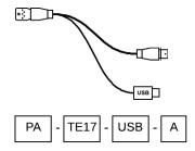
Programming adapter is used to modify configurable device parameters, retrieve cleaning cycle data, and update internal microcontroller firmware. Suitable for inline connection to TE-1700
